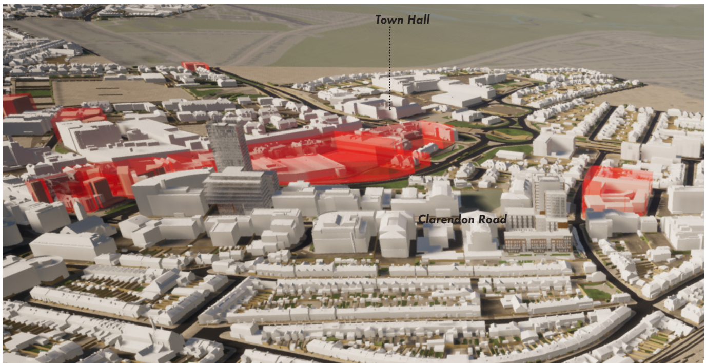
Fig 48 View looking across west across the town centre showing 5 and 8 storey height parameters in orange and automatically generated (non-designed) blocks to illustrate the scale of potential development
