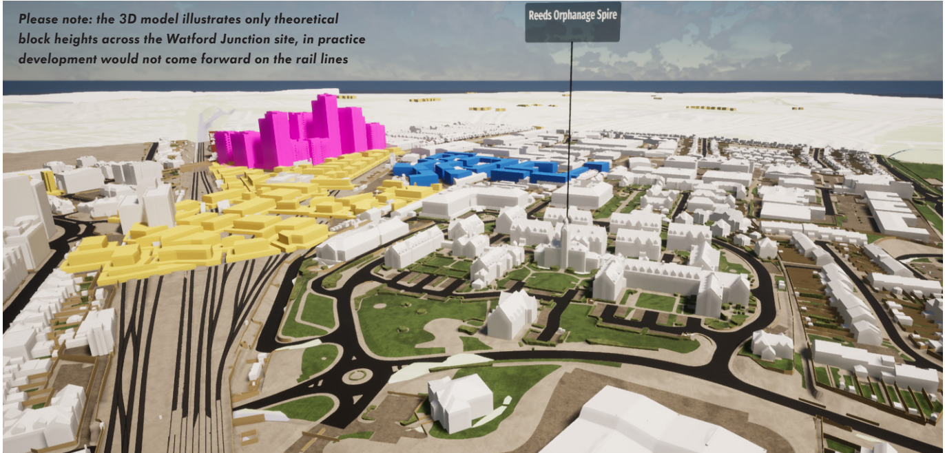
Fig 33 Baseline scenario 2 - existing prevailing heights +50%: 3D model view showing example blocks of this height uplift at Watford Gateway sites in blue and yellow (against the context of existing buildings in white, and the permitted scheme at St Albans Road in pink)
