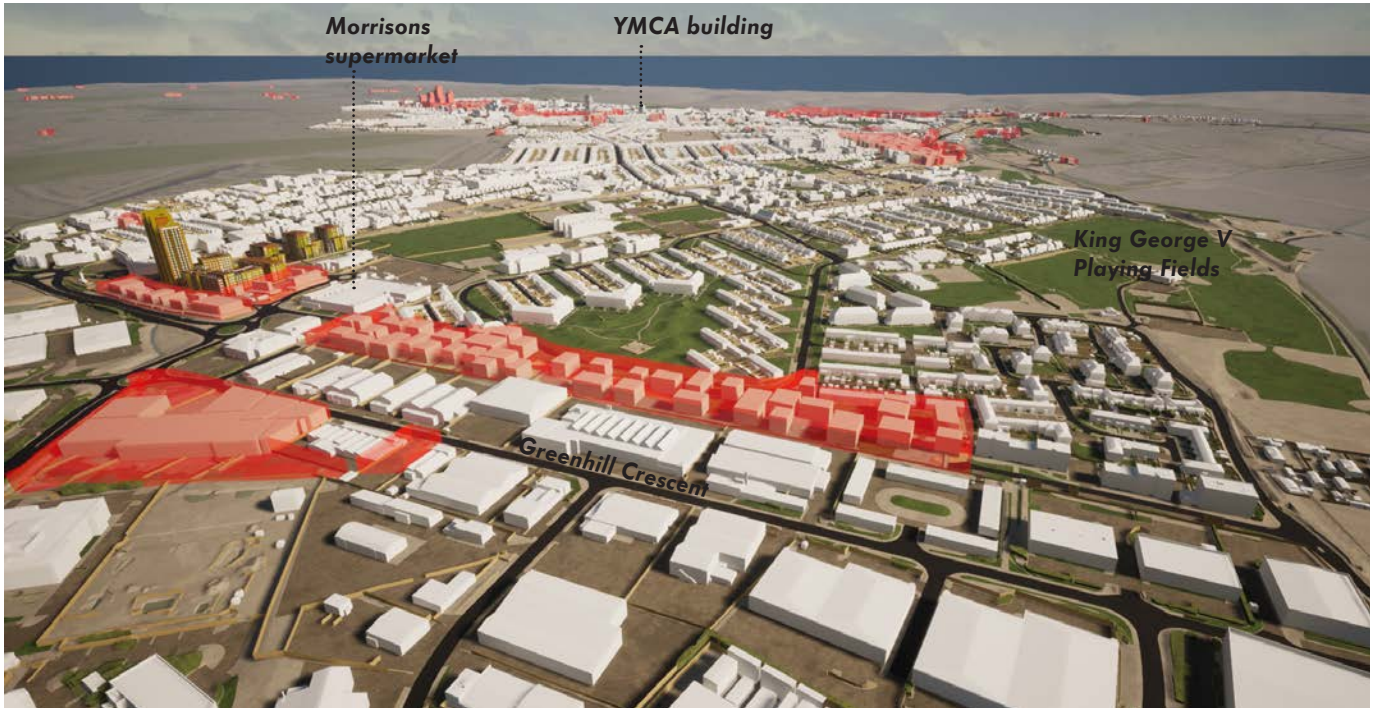
Fig 56 View looking across Ascot Road showing 4 storey height parameter in orange and automatically generated (non-designed) blocks to illustrate the scale of development
