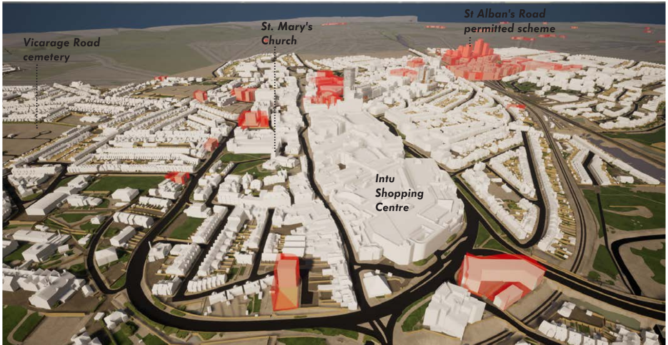
Fig 47 View looking across north across the town centre showing 5 and 8 storey height parameters in orange and automatically generated (non-designed) blocks to illustrate the scale of development
