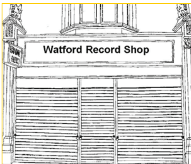
Solid shutters are not acceptable
